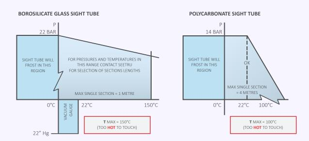
The above constraints are approved for water and other non-aggressive liquids only. For any liquid or for any constraint in excess of those given above, please consult Seetru.
