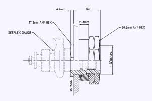
The tank boss is only suitable for use with tanks of wall thickness from 1.58mm (1/16") to 7.9mm (5/16") hole diameter of 42.0mm is required in the tank wall.
